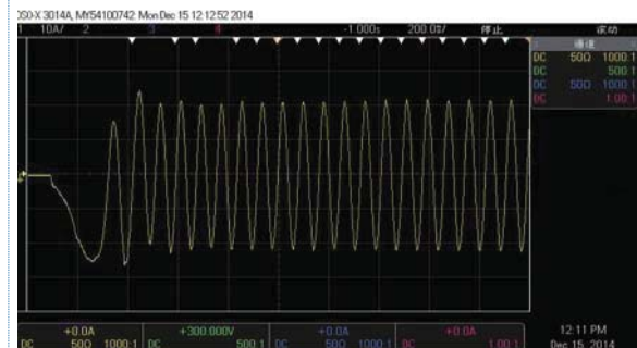
Fast startup current waveforms of 4 kW synchronous motor at 200% load
